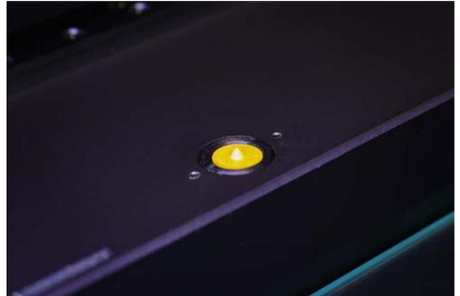
3. Using the incremental adjustment buttons, adjust the X axis nozzle position so that the tip of the nozzle is exactly above the template pointer. Press "**Adjust Y axis**" to proceed to Y axis adjustment.
