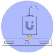
**The printing surface control system** in most cases makes it possible to detect in a timely manner if the printed model is not securely attached to the platform or if a foreign object is present when printing the current layer. If an item comes unstuck or the printed layer has the wrong shape, the printer will pause printing until the user intervenes.
