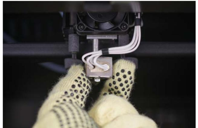
**8.** Perform the desired operation: clean the flow channel or replace the heating unit.
