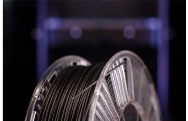
4. Open the side door and remove the filament spool. Close the side door and press "Finish".
